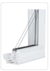
Multiple chambers increse strength and energy performance whille allowing efficient water drainage from the pocket sill. 1" oa. dual and triple pane insulated glass options and Fliplock positive action locks for security.
